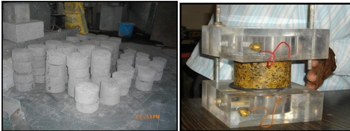
Fig.3 RCPT Test Specimen and Test arrangement
