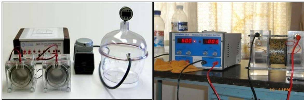
Fig.1 RCPT Test Equipment and Set Up.
